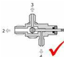
Fig C: Partially Opened Condition (5.5 turns clockwise from fully opened condition. Port 2, 3, 4 is fully opened).
