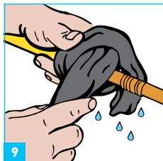
9 Wrap exposed plastic with a damp cloth
