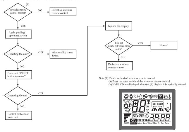
Simplified check method of wireless remote control
