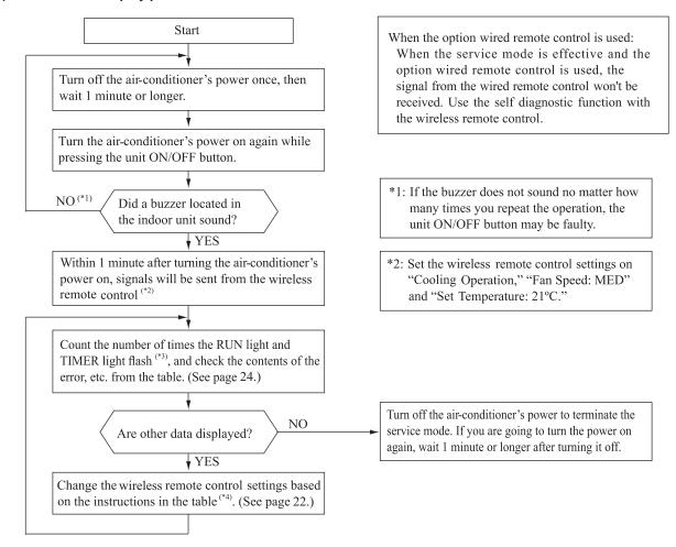
\*3: To count the number of flashes in the service mode, count the number of flashes after the light lights up for 1.5 second initially (start signal). (The time that the light lights up for 1.5 second (start signal) is not counted in the number of flashes.)
